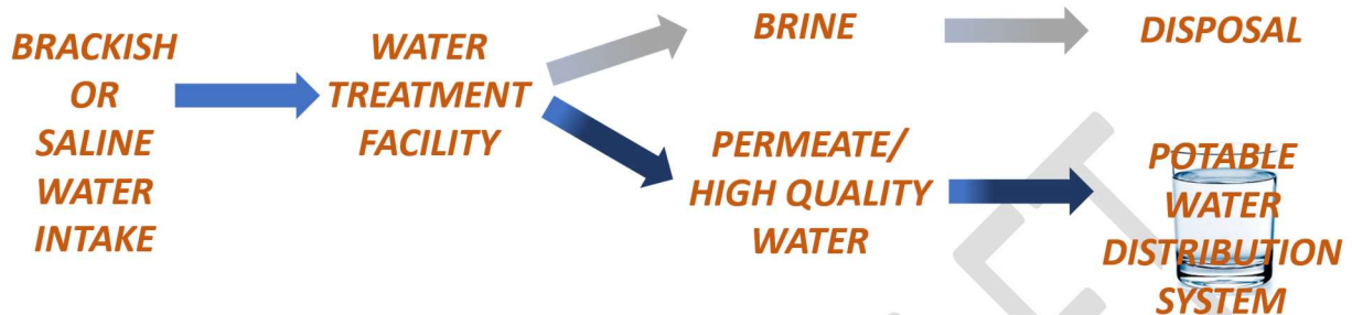
Figure 2 General Desalination Process
